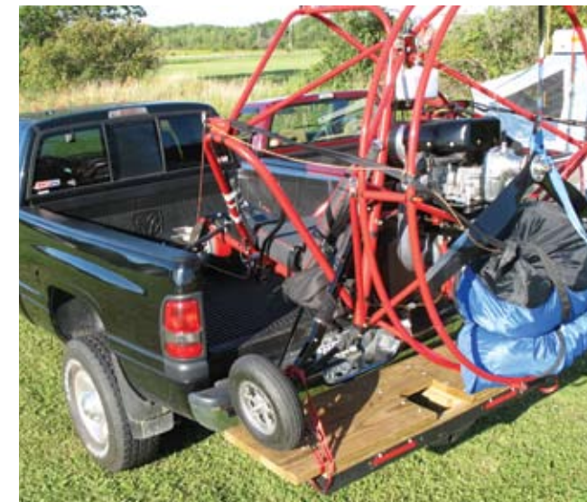
This PPC owner couldn't fit the back wheels of his machine inside the bed of his truck so he created an extension to the truck bed. Tiedown straps secure the machine to the front of the bed.
