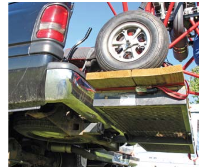
This PPC owner couldn't fit the back wheels of his machine inside the bed of his truck so he created an extension to the truck bed. Tiedown straps secure the machine to the front of the bed.
