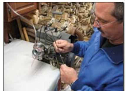
Mark Bayer examines the improvised throttle cable for the 32-mm Mikuni carburetor.
