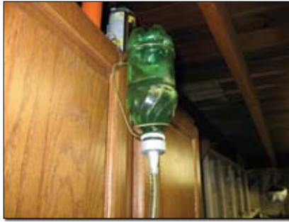
Here's the high-tech fuel system for the test setup: The Bayer brothers routed a fuel line from the makeshift fuel tank, a recycled 16-ounce soda bottle, to the Mikuni carb.
