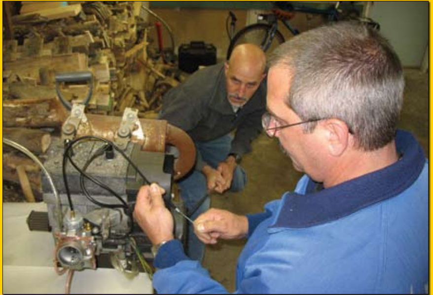
The moment of truth: Author Tim Bayer (background) pulls the start rope while Mark operates the throttle via the improvised cable.
