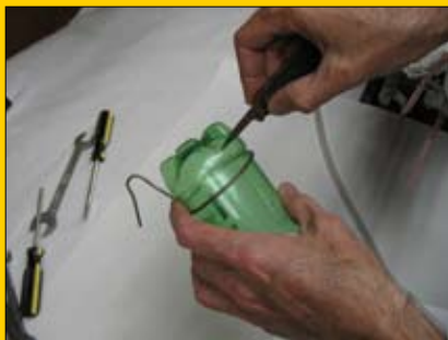
Oops! Vapor lock! A quick vent of the high-tech fuel tank solved that problem.
