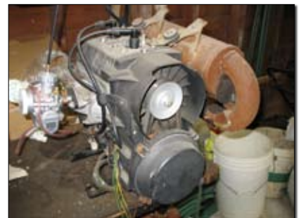
Key to the Rally project? The 35-hp Cuyuna 430 powerplant meant to power the plane. The heads and cylinders were in good condition, so it was workable.
