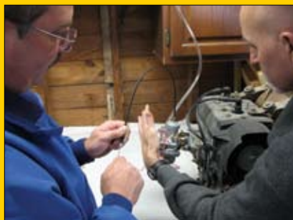
With no choke, the author used the palm of his hand to mimic the choke's operation and inhibit airflow down the barrel of the carburetor.
