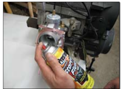
The Mikuni carb assembly did not include a choke, so the brothers resorted to pumping the carb with starting fluid.
