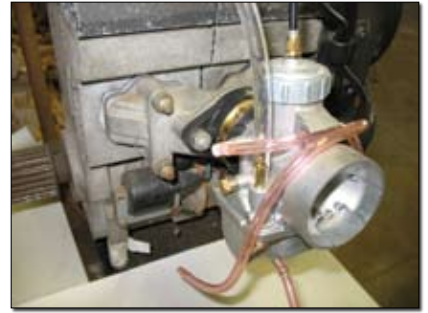
Here's the high-tech fuel system for the test setup: The Bayer brothers routed a fuel line from the makeshift fuel tank, a recycled 16-ounce soda bottle, to the Mikuni carb.
